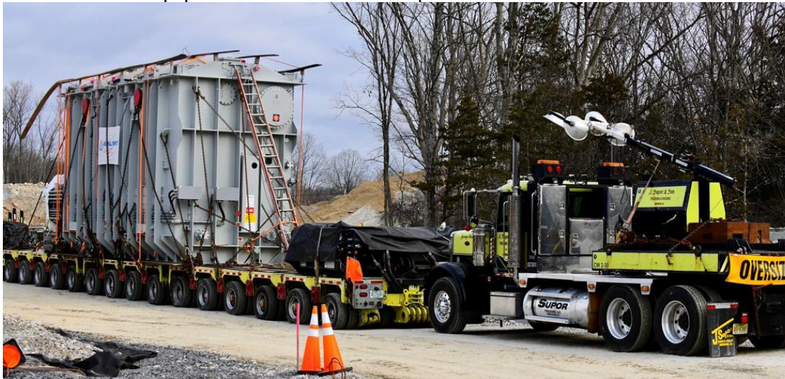
Photo 2 – PAR equipment on oversized transport truck.
